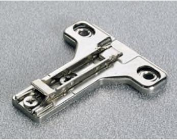
Face frame adapter mounting plates are now available in thickness of 1.0mm, 4.0mm and 6.5mm. Screw holes are placed at 10mm for centering on 19mm frame (Standard) or placed at 13mm for thicker frame (XR). Both offer a 3rd screw fixing option.
