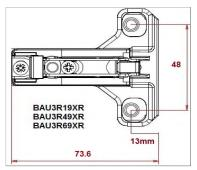
Salice is pleased to introduce two additions to our face frame adapter mounting plate series. One is the addition of a 6.5mm thick face frame mounting plate and the other is the addition of a face frame plate with a 13mm hole position.
