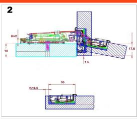
17.5mm overlay Hinge: Full overlay (A type) 2.0mm mounting plate: BARGR29/16 K = 4.5mm
