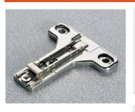
Face frame adapter mounting plates are now available in thickness of 1.0mm, 4.0mm and 6.5mm. Screw holes are placed at 10mm for centering on 19mm frame (Standard) or placed at 13mm for thicker frame (XR). Both offer a 3rd screw fixing option.
