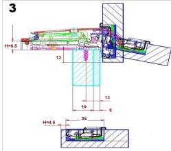
13mm overlay Hinge: Full overlay (A type) 6.5mm mounting plate: BAU3R69XR K = 4.5mm
