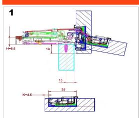
13mm overlay Hinge: Full overlay (A type) 6.5mm mounting plate: BAU3R69 K = 4.5mm
