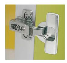
**Salice Short Arm** Series 300 Concealed hinge, 45mm operating profile. 94° opening angle, 11mm deep metal cup, 35mm cup dia.
