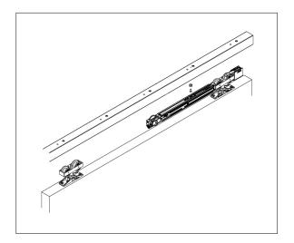
The SoftMove soft-closing mechanism is an accessory for all Hawa-Junior 40-80-120 systems suitable for both wood and glass sliding doors. The mechanism is completely integrated into the upper running track. The SoftMove soft-closing mechanism gently decelerates sliding doors and draws them into their final position. Quick and easy to install with included installation aids. Uses a high quality hydraulic damper that is very quiet, with long lasting and maintenance free materials.
